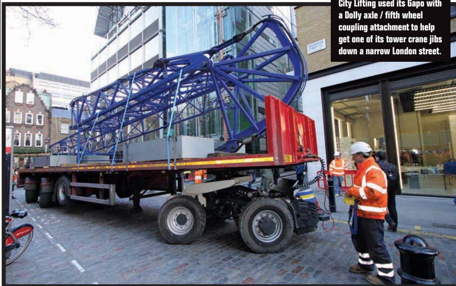
The clever combination of the Gapo and the rear steer trailer was able to deliver the crane jib around the tight bend.
